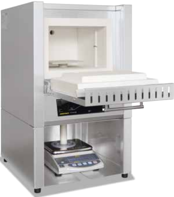
Weighing furnace L 9/11/SW with flap door
