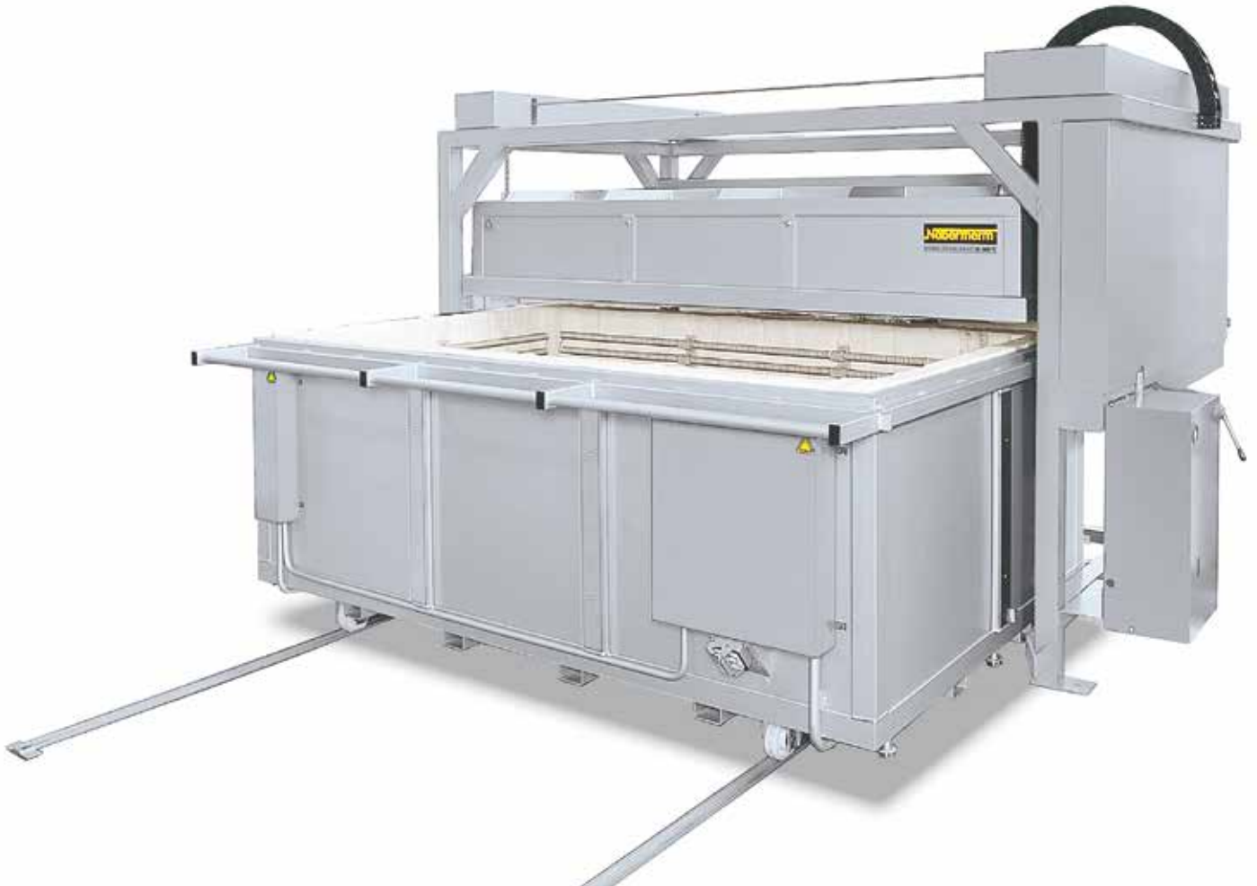
Top hat furnace GW 2208/S with electro-hydraulically driven hood, tub can be pulled out on rails
