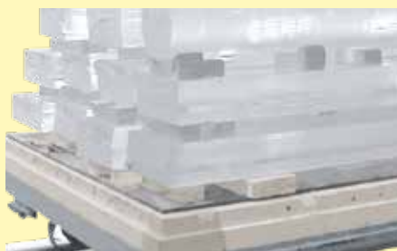
Bogie hearth furnace for tempering quartz rods
