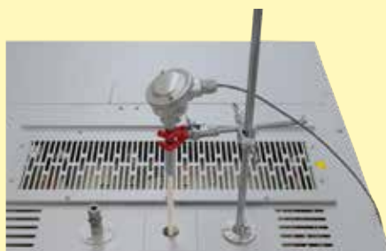
Thermocouple port in the ceiling with tripod
