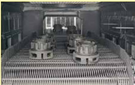
Mesh belt drive in a continuous furnace
