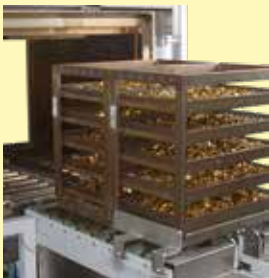
Continuous furnace for bulk materials in baskets
