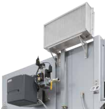
Direct gas-firing at a chamber oven
