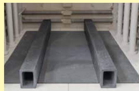
SiC support beams for ease of loading/unloading using a forklift
