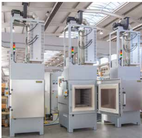
Production plant with three forced convection chamber furnaces NA 250/85 DB200 for debinding and catalytic post combustion system KNV 320 (reduced footprint construction)
