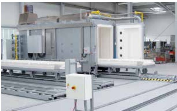
Gas-fired bogie hearth furnace WB 6200/12 BO for burning out ceramic insulating materials
