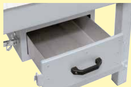
Drawer for collection of liquid wax
