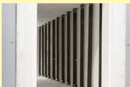
SiC rod elements on both sides of the bogie hearth furnace
