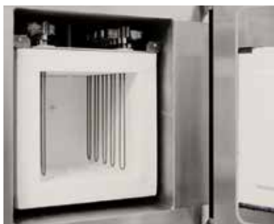
Molybdenumdisilicide heater and fiber insulation
