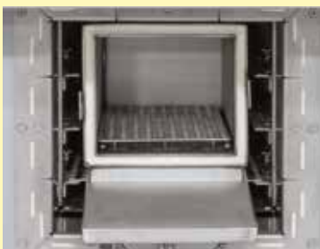
Protective gas box which stays in the furnace
