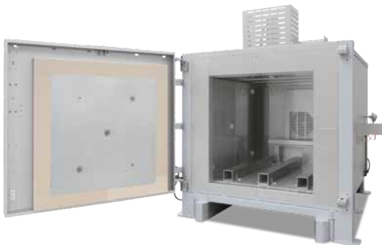
Forced convection chamber furnace NA 1500/45 on base with guide rails and end stop for a custom-built charging forklift, custom-built charge support and ramming protection
