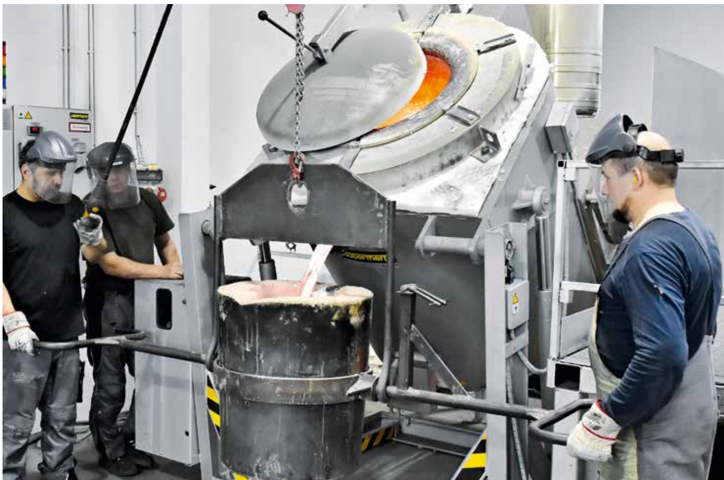
Tilting furnace KB 150/12 in production
