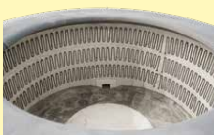
Meander heating elements
