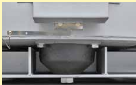
Forklift entry with dampers
