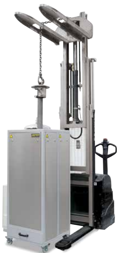
Cleaning furnace SRO 170/1000/11 with suspended pipe
