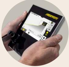
Recording of firing data of the connected controller via USB stick
