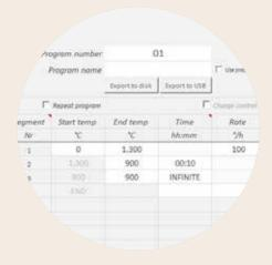
Firing data input via NTEdit software (freeware) for MS Windows<sup>TM</sup>
