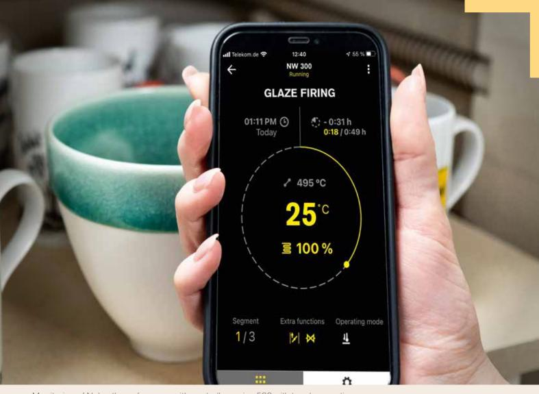
Monitoring of Nabertherm furnaces with controller series 500 with touch operation
