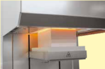
Electrically driven lift-bottom
