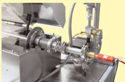
Gas tight rotating union with gas cooler and charge thermocouple
