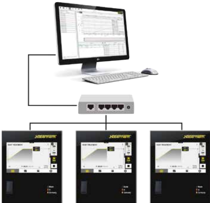
Example lay-out with 3 furnaces
