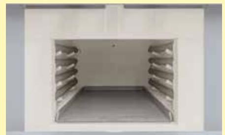
Deep furnace chamber with three-sides heating
