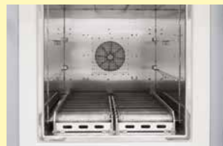
Roller conveyor in furnace chamber
